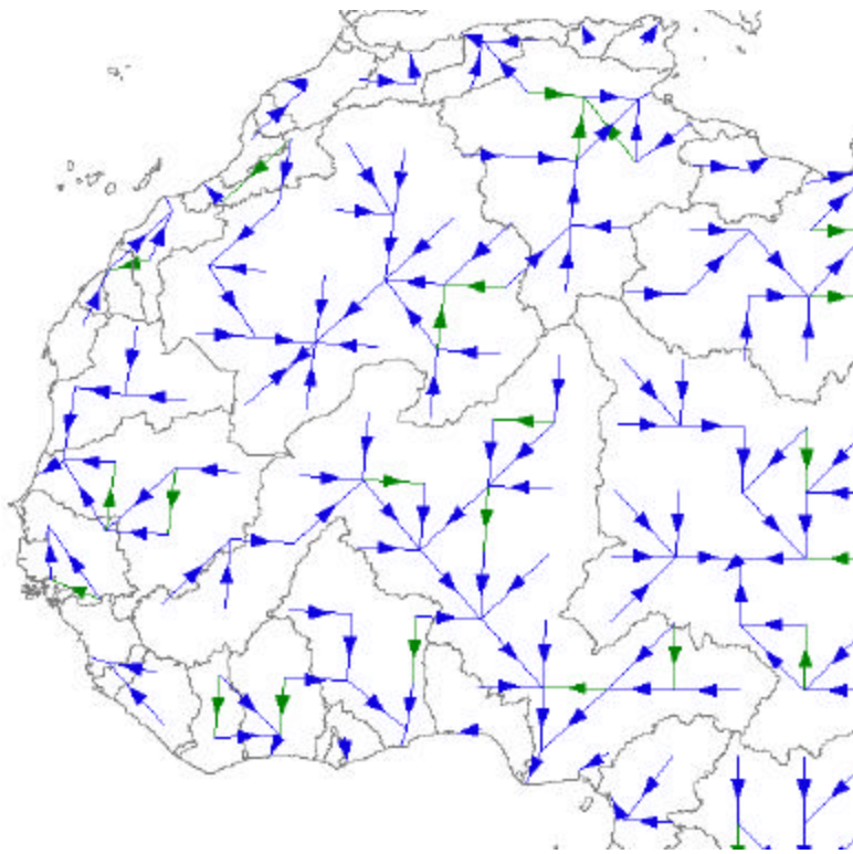
Figure 4.12 Manual (Green) and Double Maximum (Blue) River Networks with the West African Watersheds
