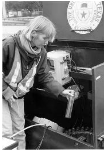
(b) The storm water sampling station
