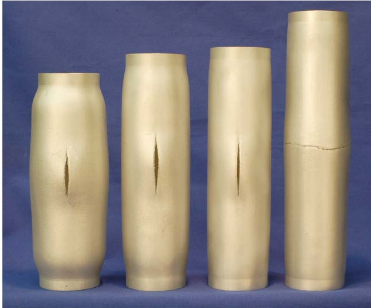
Fig. 3.7 – A set of failed specimens tested at different biaxiality ratios: from left to right, \alpha = -0.2, 0, 0.75, 1.0
