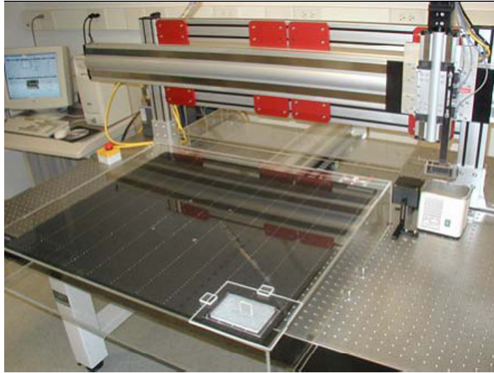
Figure 2-7: A custom built DNA microarray printing robot.
