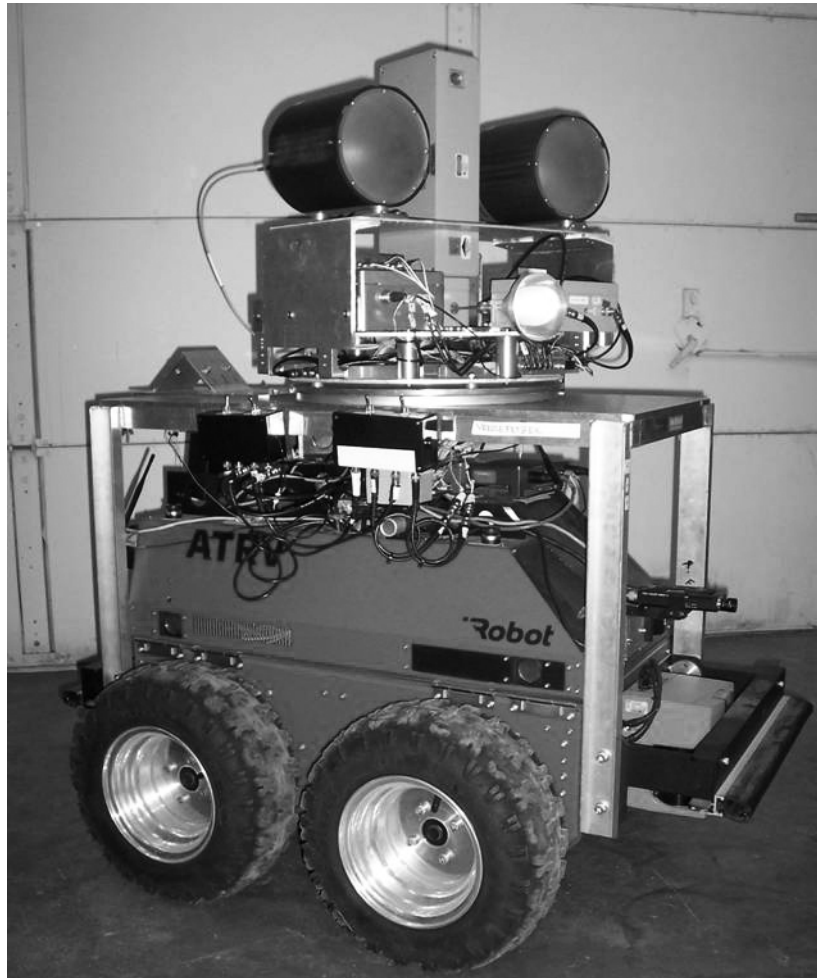
Figure 4.1. Correlation radiometer atop the mobile platform. The black antennas feed the K a -band radiometer.
