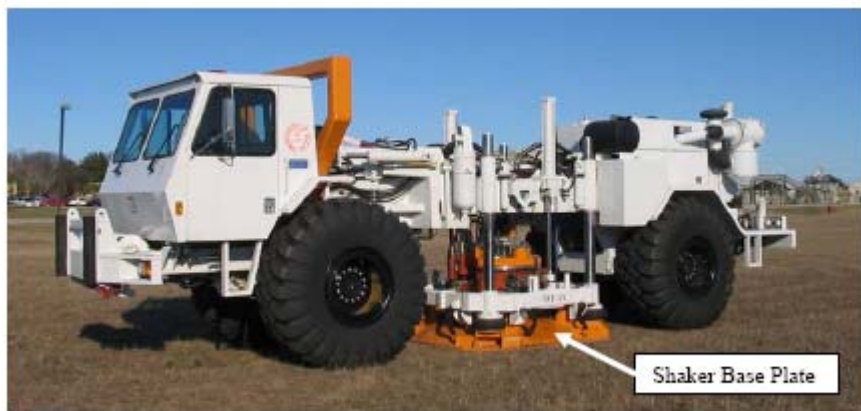
Figure 3.1 Tri-axial vibrator: T-Rex (from Stokoe et al, 2004)
