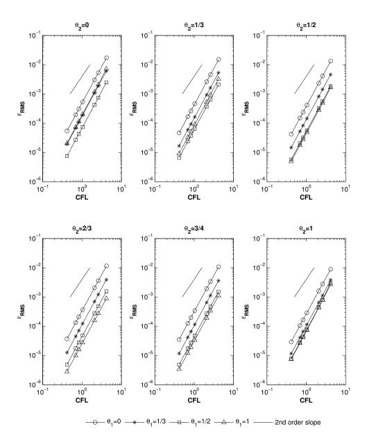
Figure 5.2 Temporal accuracy of various combinations of  $\theta_2$  and  $\theta_1$  for solution of the Burgers' equation at t=0.6, where  $\Delta x = 1/50$ ,  $\nu = 0.05$  and  $\Delta t = 0.6/\Gamma$  ( $\Gamma \in \{5, 8, 10, 20, 25, 30, 50\}$ ).
