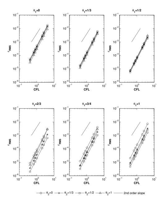
Figure 5.1 Temporal accuracy of various combinations of  $\theta_1$  and  $\theta_2$  for solution of the Burgers' equation at t=0.6, where  $\Delta x = 1/50$ , v = 0.05 and  $\Delta t = 0.6/\Gamma$  ( $\Gamma \in \{5, 8, 10, 20, 25, 30, 50\}$ ).
