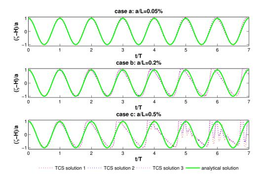
Figure 6.3 Simulations in the inviscid flow with different wave steepness
