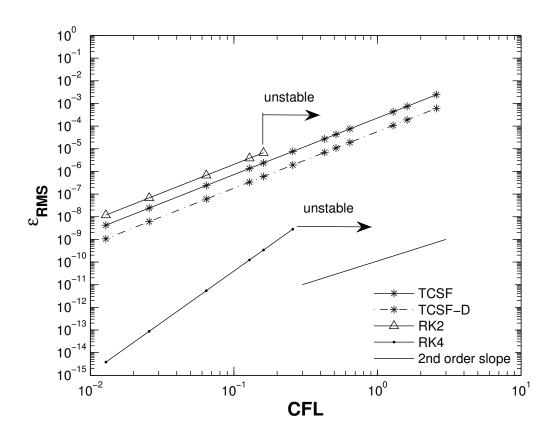
Figure 4.6  $\epsilon_{RMS}$  vs. CFL number of TCSF, RK2 and RK4 methods for solution of 1D conservative Burgers' equation, where  $\nu = 0.05$   $\Delta x = 1/50$ , and  $\Delta t = 0.3/\Gamma$  with  $\Gamma \in \{500, 200, 100, 80, 50, 30, 25, 20, 10, 8, 5\}$ .
