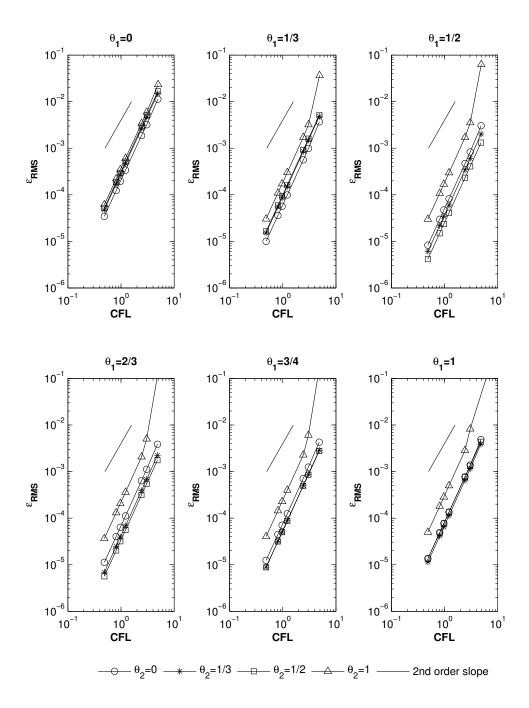
Figure 5.4 Temporal accuracy of various combinations of  $\theta_2$  and  $\theta_1$  for solution of the Burgers' equation at t=1, where  $\Delta x = 1/50$ ,  $\nu = 0.05$  and  $\Delta t = 1/\Gamma$  ( $\Gamma \in \{5, 8, 10, 20, 25, 30, 50\}$ ).
