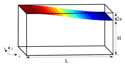
Figure 6.2 A standing wave in a rectangular basin
