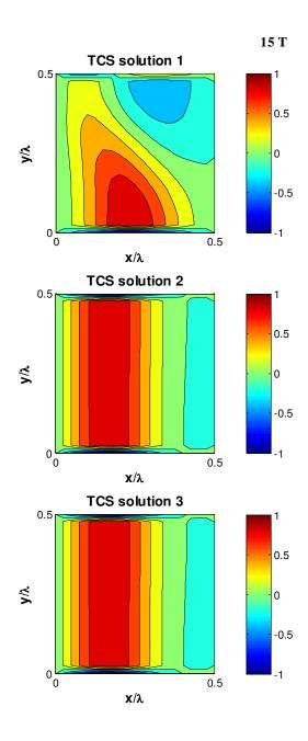
Figure 6.10 Normalized U-velocity contours in the computational domain at time 15T.
