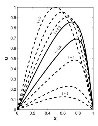
Figure 4.1 Solution of 1D Burgers' equation evolving in time for  $t \in \{0, 0.1, 0.2, 0.3, 0.6, 1, 2, 3\}$  using v = 0.05 along with the initial and boundary conditions of Equations (4.43) through (4.45).
