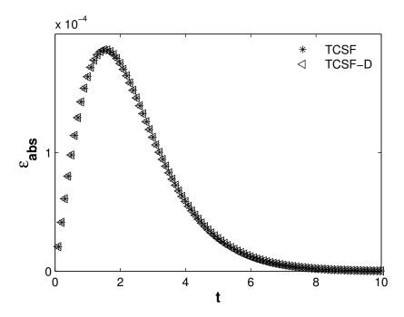
Figure 4.14 Time evolution of absolute errors for TCS methods applied to the ODE, Equation (4.101), for  $\Delta t$  =0.1, where  $\epsilon_{abs}(t) = \left| y_{model}(t) - y_{analytical}(t) \right|$ .
