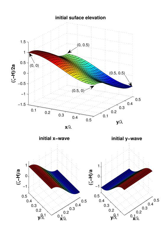
Figure 6.5 The initial 2D standing wave and its decomposed x and y direction 1D wave
