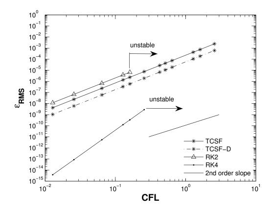
Figure 4.12 Temporal accuracy of the TCS and RK methods for solution of 1D non-conservative Burgers' equation at different CFL numbers, where  $\nu$ =0.05,  $\Delta x$  =1/50 and  $\Delta t$  =0.6/ $\Gamma$  with  $\Gamma$   $\in$  {500, 200, 100, 80, 50, 30, 25, 20, 10, 8, 5}.
