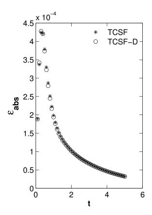
Figure 4.2 Absolute error time evolution for numerical solutions of 1D conservative Burgers' equation for TCSF and TCSF-D using {  $\Delta t = 0.01$ ,  $\Delta x = 1/50$ ,
