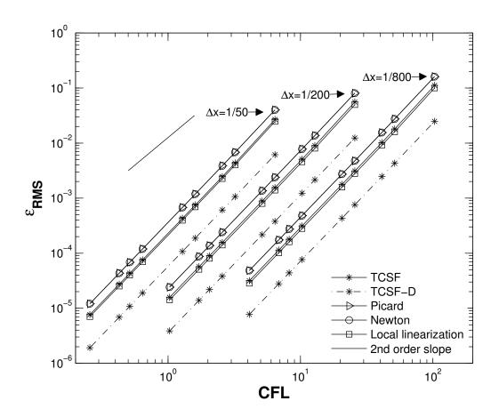
Figure 4.3  $\epsilon_{RMS}$  vs. CFL number of various methods for solution of 1D conservative Burgers' equation with three different  $\Delta x$ , where  $\nu=0.05$  and  $\Delta t=0.3/\Gamma$  with  $\Gamma\in\{50,\,30,\,25,\,20,\,10,\,8,\,5,\,4,\,2\}$ .
