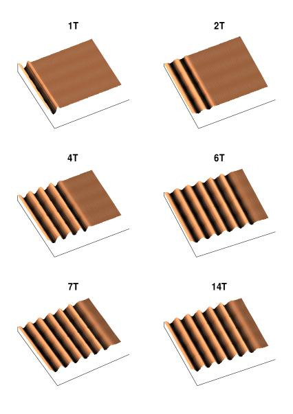
Figure A.10 Time evolution of a progressive wave at different wave periods from TCS solution 1.
