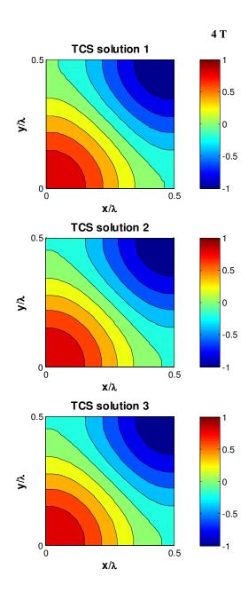
Figure 6.7 Normalized surface elevation contours in the computational domain at time 4T.
