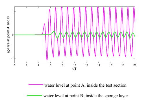
Figure A.7 Water level evolutions inside the test section and sponge layer.
