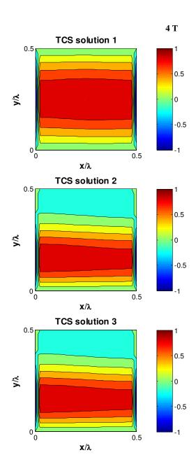
Figure 6.11 Normalized V-velocity contours in the computational domain at time 4T.
