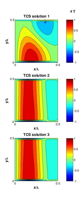
Figure 6.9 Normalized U-velocity contours in the computational domain at time 4T.
