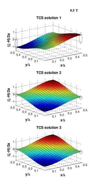
Figure 6.14 Snapshot of the standing wave at 0.5 T. The surface displacements at the two monitored points (0.5, 0) and (0, 0.5) are circled.
