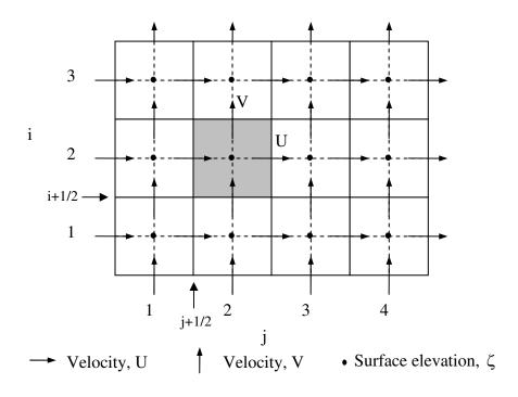
Figure 6.1 Illustration of Arakawa C grid.
