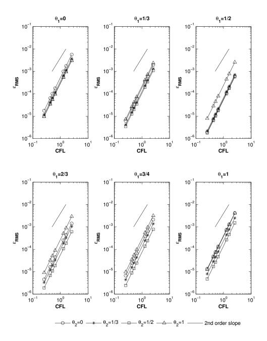
Figure 5.3 Temporal accuracy of various combinations of  $\theta_2$  and  $\theta_1$  for solution of the Burgers' equation at t=0.3, where  $\Delta x = 1/50$ ,  $\nu = 0.05$  and  $\Delta t = 0.3/\Gamma$  ( $\Gamma \in \{5, 8, 10, 20, 25, 30, 50\}$ ).
