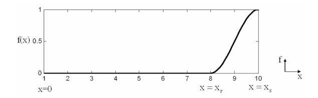
Figure A.3 Shape function of viscosity
