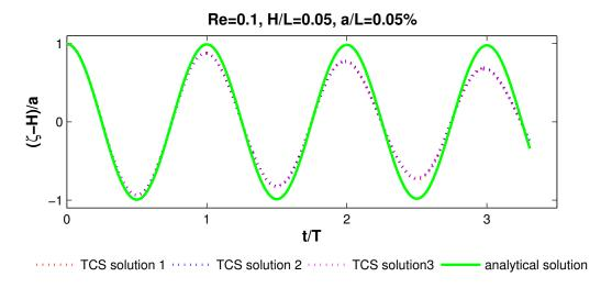
Figure 6.4 Viscous damping effects in the shallow water model
