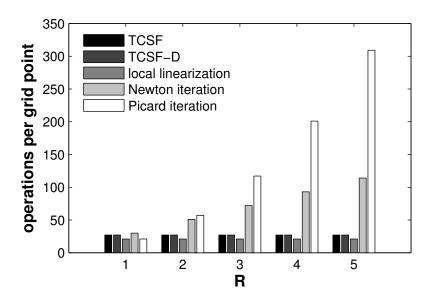
Figure 4.7 Ideal operations per grid point for one time step using various nonlinear solution methods for 1D conservative Burgers' equation. R is the number of outer iterations taken by Newton method. It is assumed that the Picard method convergences in R<sup>2</sup> outer iterations.
