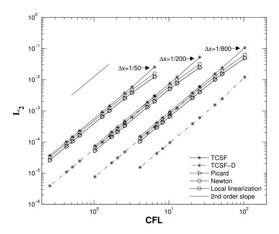
Figure 4.4  $L_2$  norm vs. CFL number of various methods for solution of 1D conservative Burgers' equation with three different  $\Delta x$ , where  $\nu=0.05$  and  $\Delta t=0.3/\Gamma$  with  $\Gamma\in\{50,30,25,20,10,8,5,4,2\}$ .
