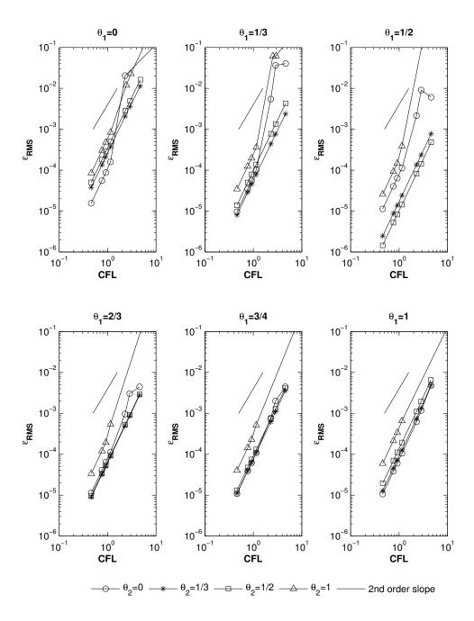
Figure 5.5 Temporal accuracy of various combinations of  $\theta_2$  and  $\theta_1$  for solution of the Burgers' equation at t=2, where  $\Delta x = 1/50$ ,  $\nu = 0.05$  and  $\Delta t = 2/\Gamma$  ( $\Gamma \in \{5, 8, 10, 20, 25, 30, 50\}$ ).
