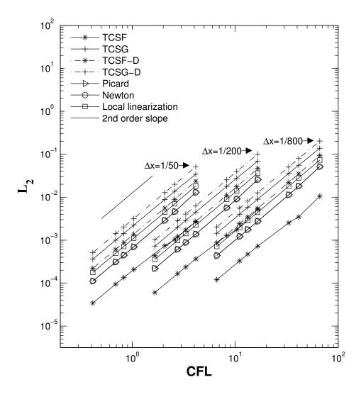
Figure 4.10  $L_2$  norm vs. CFL numbers of various methods for solution of 1D non-conservative Burgers' equation at different CFL numbers, where v=0.05,  $\Delta x$  =1/50 and  $\Delta t$  =0.6/ $\Gamma$  with  $\Gamma$   $\in$  {50, 30, 25, 20, 10, 8, 5}.
