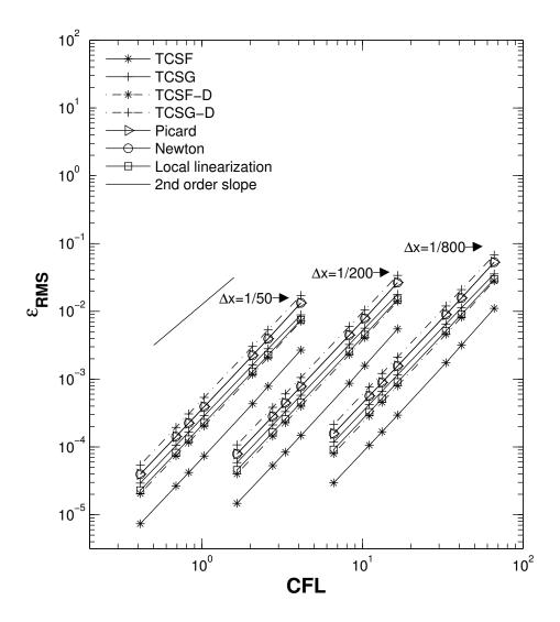
Figure 4.9  $\epsilon_{RMS}$  vs. CFL numbers of various methods for solution of 1D non-conservative Burgers' equation at different CFL numbers, where  $\nu$ =0.05,  $\Delta x$  =1/50 and  $\Delta t$  =0.6/ $\Gamma$  with  $\Gamma$   $\in$  {50, 30, 25, 20, 10, 8, 5}.
