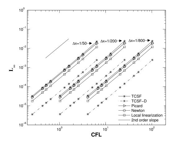
Figure 4.5  $L_{\infty}$  norm vs. CFL number of various methods for solution of 1D conservative Burgers' equation with three different  $\Delta x$ , where  $\nu=0.05$  and  $\Delta t=0.3/\Gamma$  with  $\Gamma\in\{50,\,30,\,25,\,20,\,10,\,8,\,5,\,4,\,2\}$ .
