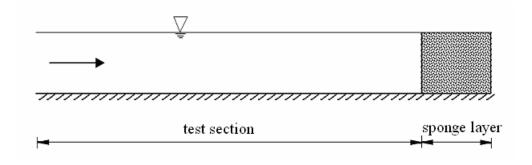
Figure A.4 An open boundary rectangular channel with a sponge layer
