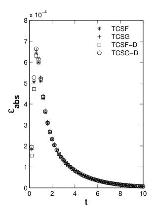
Figure 4.8 Absolute error time evolution for numerical solutions of 1D non-conservative Burgers' equation for the TCSF and TCSG methods using  $\left\{\Delta t = 0.01, \, \Delta x = 1/50, \, v = 0.05\right\} \text{ where}$   $\varepsilon_{abs}(t) = \left|\frac{1}{50}\sum_{i=1}^{50}u_{model}(x_i,t) - u_{analytical}(x_i,t)\right| \text{ and } u_{analytical}(x,t) \text{ is numerically}$
