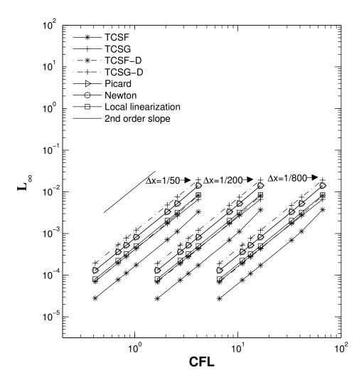
Figure 4.11  $L_{\infty}$  norm vs. CFL numbers of various methods for solution of 1D non-conservative Burgers' equation at different CFL numbers, where  $\nu$ =0.05,  $\Delta x$  =1/50 and  $\Delta t$  =0.6/ $\Gamma$  with  $\Gamma$   $\in$  {50, 30, 25, 20, 10, 8, 5}.
