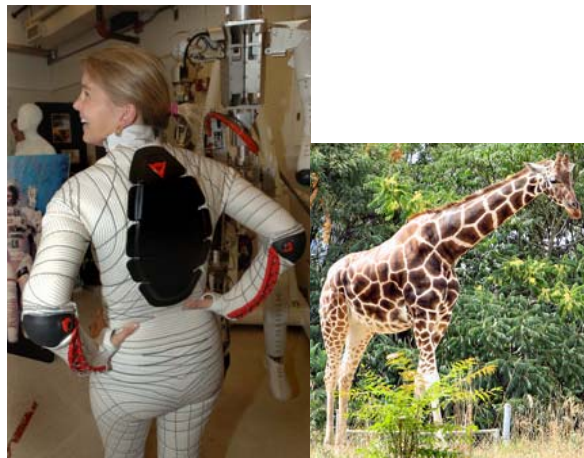
Figure 4: The ultra maneuverable and lightweight space suit, partially inspired by the tight skin of a giraffe's legs which helps to regulate blood pressure, relies on mechanical pressure rather than gas pressure to support human life in a thin atmospheric environment like mars ("A Clothes Encounter", 2007).
