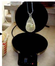
The whisk adheres to the batter while it is translated to the waffle iron.
