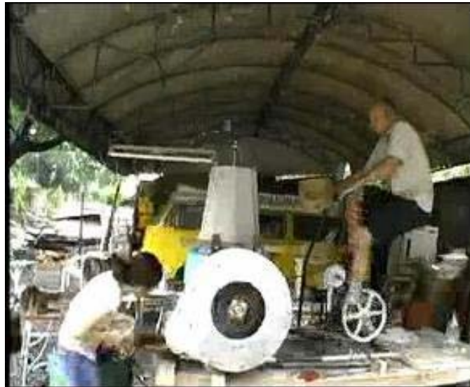
Figure 92: A search result from the control condition for an existing peanut shelling machine for developing countries (“The Appropriate Genius: Documentary,” 2007). This machine uses the same shell removing mechanism as the hand-powered device and also separates the shells and the nuts.
