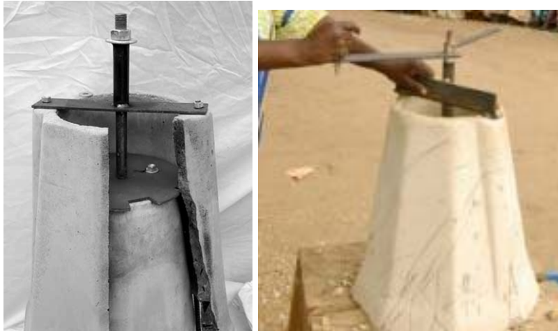
Figure 91: Participants in the control group only found within domain solutions to the peanut shelling problem. This solution is a hand-powered device that removes the shell from the peanuts (“Full Belly Project”, 2006).
