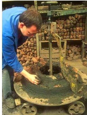
Figure 73: A stickle is used in the process of creating a bell. A stickle smooths the inner and outer surface of a bell (Putman, 1970, http://www.cccbr.org.uk/prc/pubs/slides/16startingCore.jpg ).
