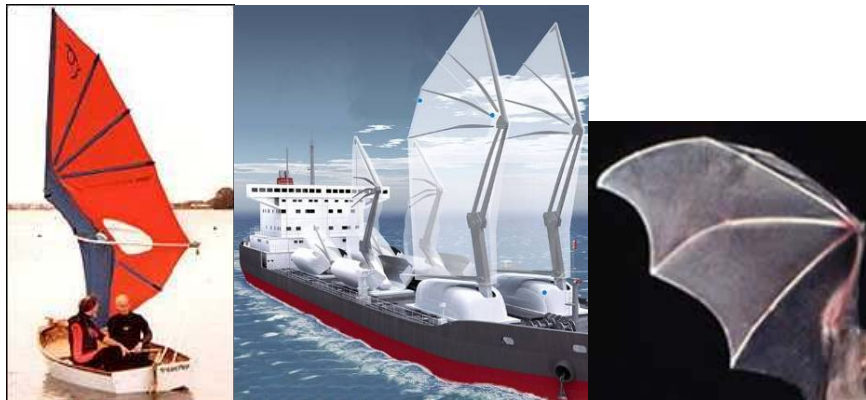
Figure 3: The sails of this cargo ship are designed based on an analogy to a bat's wing ("Wings Take to the Water," 2000; Reed, 2006; bat wing image: "El Yunque National Forest – Wildlife Facts," 2007).
