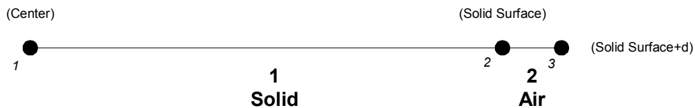
Figure 4.2: Mesh structure for 1D code
