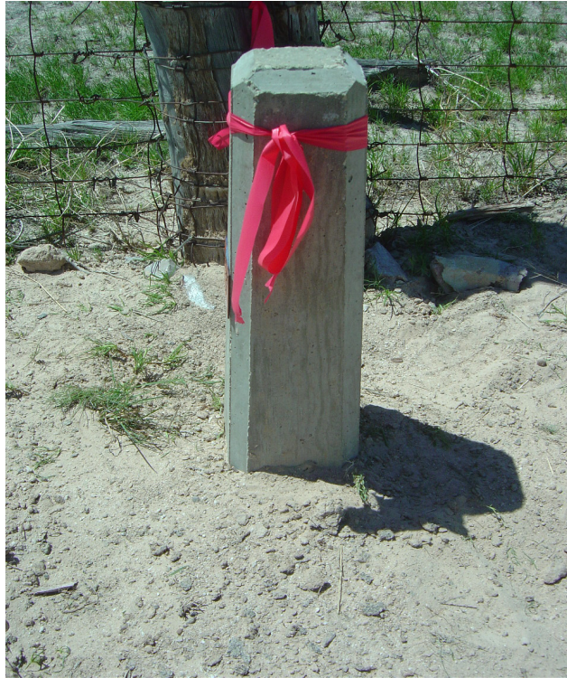
Figure 5-16: New ROW marker with Class C fly ash at 0.4 w/cm after 3 months of exposure in gypsiferous soils
