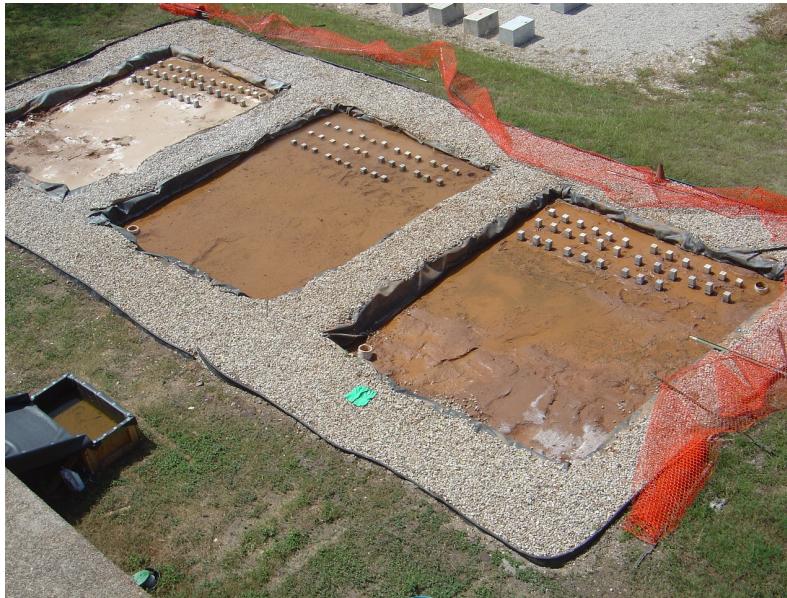
Figure 4-1: Outdoor sulfate exposure site located in Austin, TX. From left to right, the trenches contain calcium sulfate, sodium sulfate and magnesium sulfate.
