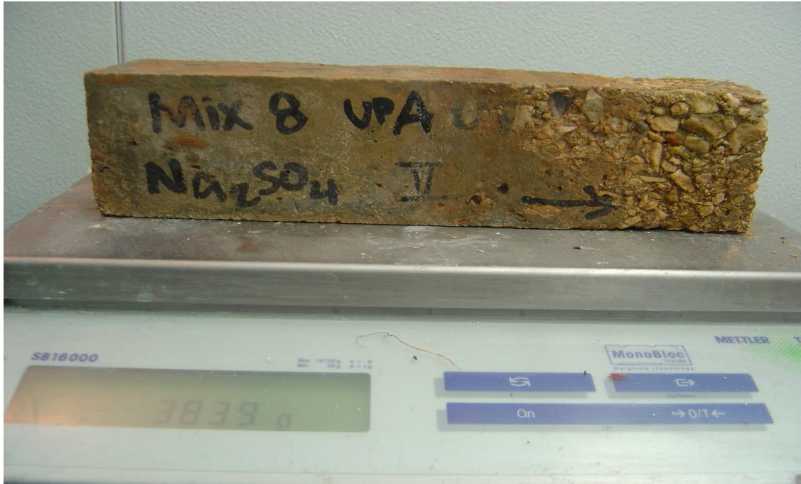
Figure 4-13: Mixture C5-7 after 18 months of outdoor exposure to sodium sulfate. This prism was placed vertically, with the section on the left fully submerged below sulfate-saturated soil.
