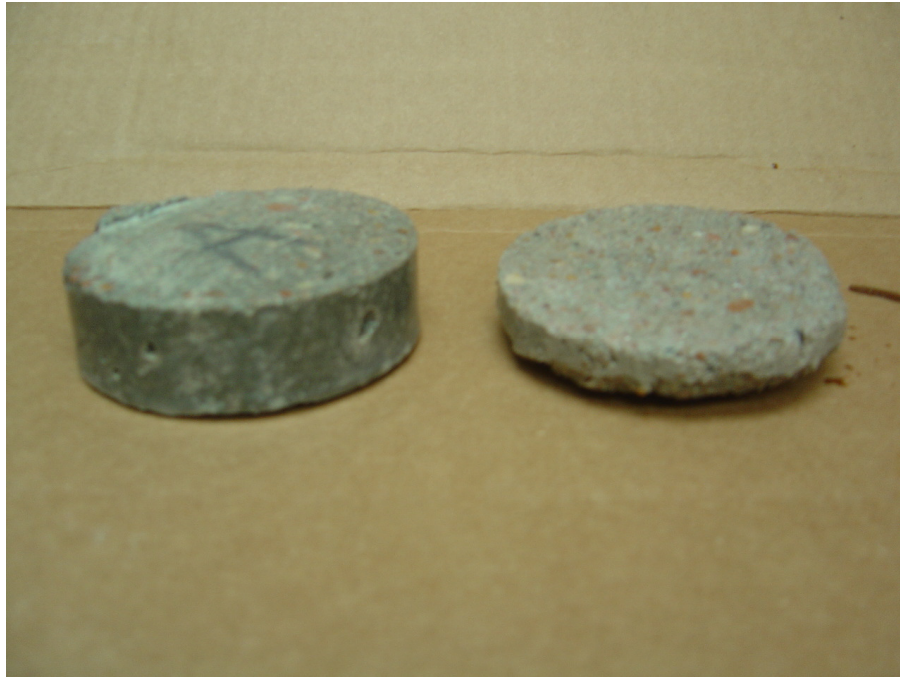
Figure 4-25: Mortar specimens before and after physical sulfate testing. The mixture contained Type V cement at 0.7w/cm. The disk on the left was prior to testing and the disk on the right went through 150 cycles.
