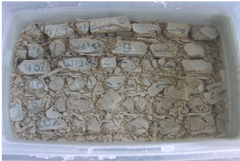
Figure 3-4: Mortar Mixture with 40% FA8 after 56 days in ASTM C 1012 testing
