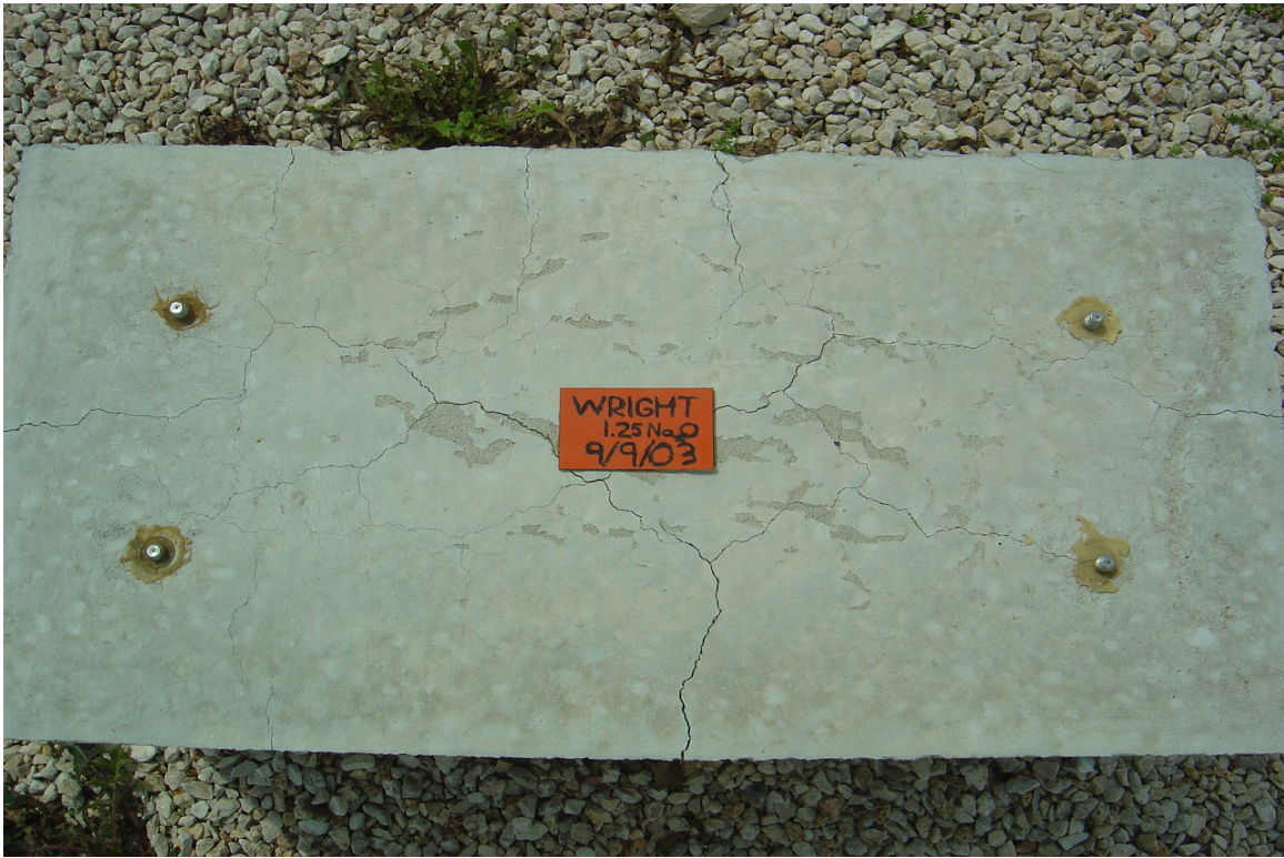
Figure 2-3: Exposure block containing highly-reactive aggregate showing less cracking after 3 years
