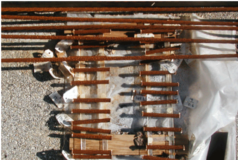
(b) Specimens after first month exposed to salt water
