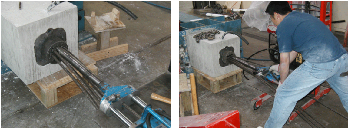
Figure 5.5 Initial Prestressing Procedure
