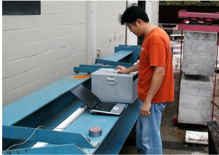
Figure 5.28 Natural Frequency Measurement of Tendon 02
