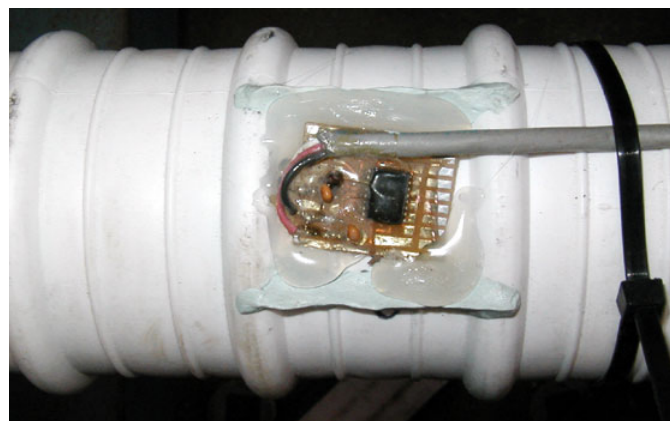
Figure 5.14 Accelerometer Attached to Tendon 01
