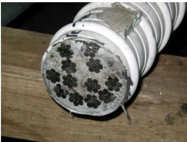
(c) Free length at north end of specimen
