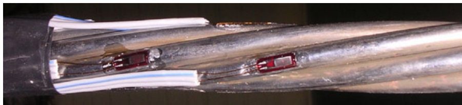
Figure 3.17 Strain Gages Positioned along Longitudinal Axes of Wires
