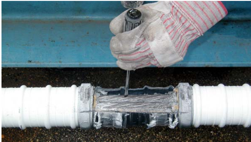
Figure 5.34 Screwdriver Penetration Test
