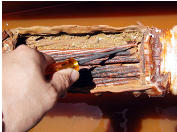
(h) Visual observation of broken wire
