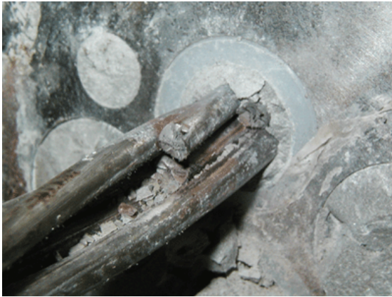
(a) Outside of anchor head (Top strand)
