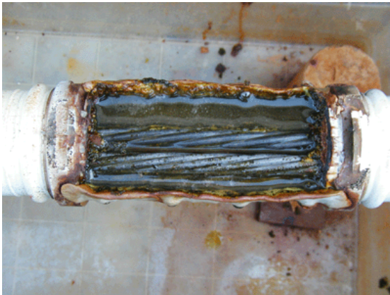
(g) Void filled with acid
