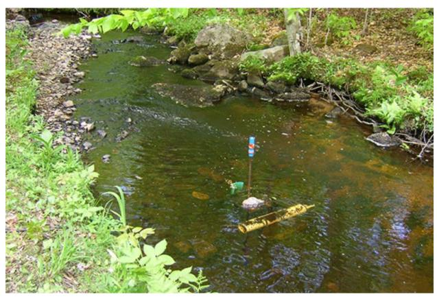
HIGH-FREQUENCY WATER QUALITY SENSOR TECHNOLOGY INSTALLED AT DOWST-CATE
