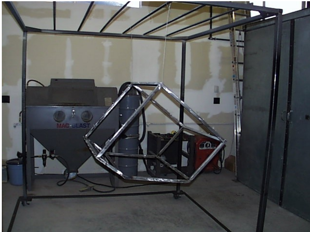
Figure 6. Frame of box prior to powder coating
