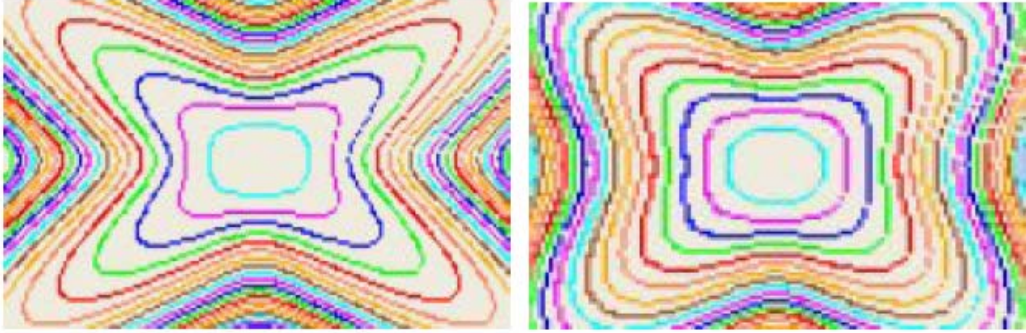
Figure 4-3: The first band E - \mathbf{k} dispersion in k_{//} plane. (left) [100] uniaxial tensile stress, (100) plane; (right) [110] uniaxial tensile stress, (110) plane, spanned by [001] and [1\bar{1}0] axes.
