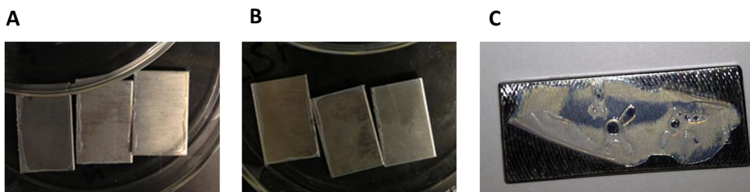
Figure 4. Digital images of the films after release study: A) PIB-PTX-COOH ; B) PIB-PS-PTX-COOH ; C) SIBS with 8.8 wt% PTX.
