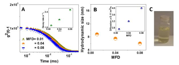
**Figure 3.** Dynamic light scattering behaviour as a function of MFD. A) Auto-correlation function of microemulsions versus time for different MFD values (inset: decay rate vs MFD); B) Hydrodynamic diameter as a function of MFD (inset: the Diffusion Coefficient versus MFD for microemulsions); C) Digital photograph of the microemulsion solution after standing for 6 months.
