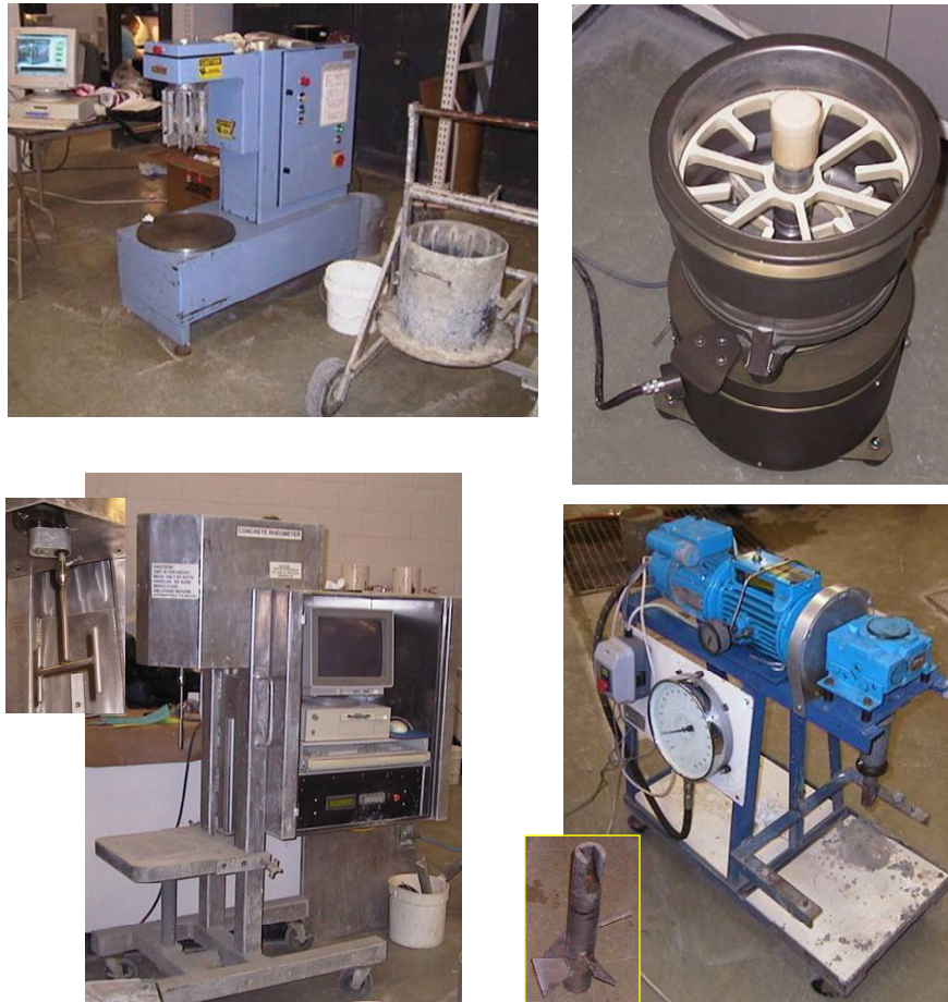
Figure 3.15: Concrete Rheometers (Clockwise from Top Left): BML, BTRHEOM, Tattersall, and IBB
