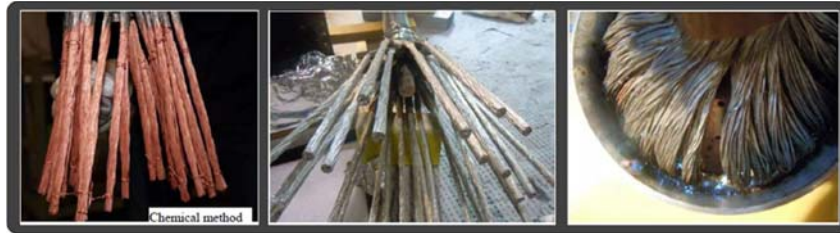
Figure 3. Preparing the sub-cables (TF-type): Left: chemical Ni removal, Middle: pre-tinning, Right: soldering into the shunt blind holes.
