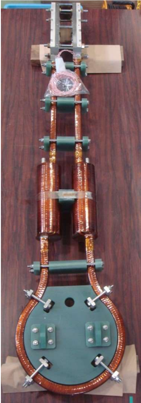
Fig. 31 Photograph of the pancake and terminal joint sample for the EF coil.
