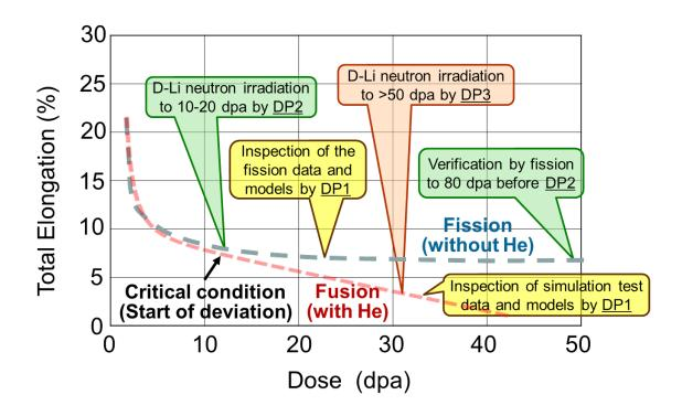
Figure 4. The role of fission and D-Li neutron irradiations for quantifying the materials degradation in the fusion condition. (Modified from Ref. 14.)
