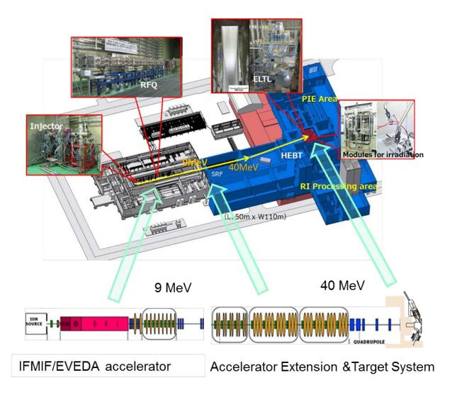
Figure 3. A schematic view of A-FNS<sup>5,13</sup>. Photographs of the facilities developed in the IFMIF/EVEDA Project are also shown
