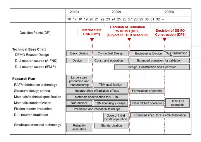
Figure 1. Technical Base Chart and Research Plan for RAFM development constructed based on the Reports and the Action Plan<sup>1-4</sup>.
