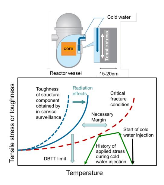
Figure 5. An illustration of the procedure to determine acceptable DBTT limit for Reactor Pressure Vessel (RPV)<sup>16</sup>.
