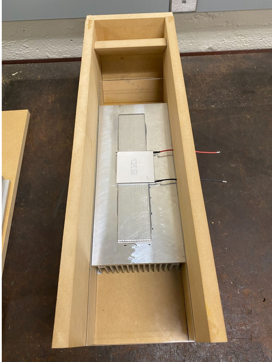
Figure 5.10: Top view of second prototype with upper hot heat sink and top panel removed.
