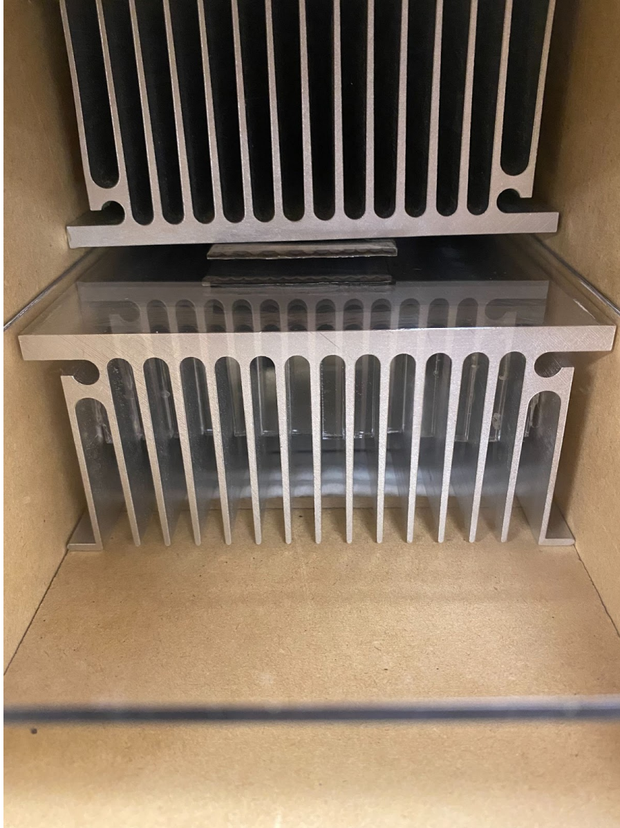
Figure 5.11: Close up view of division between upper and lower channel with view of wicking material under the fins of the cold heat sink.
