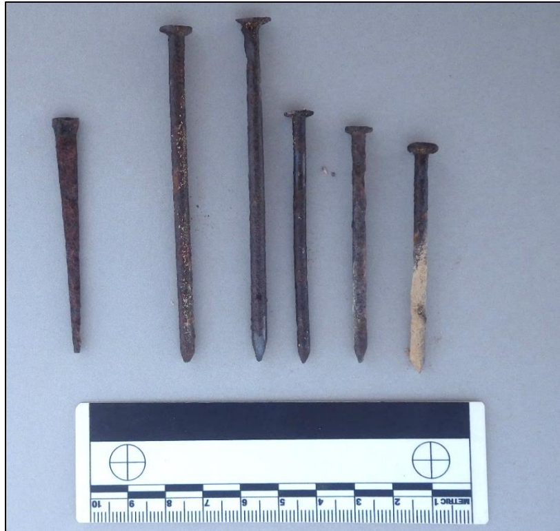
Figure 26. Sample of nails encountered at the site. From left to right: one 9D square-cut nail, two 20D wire nails, one 10D wire nail, one 9D wire nail, and one 8D wire nail.
