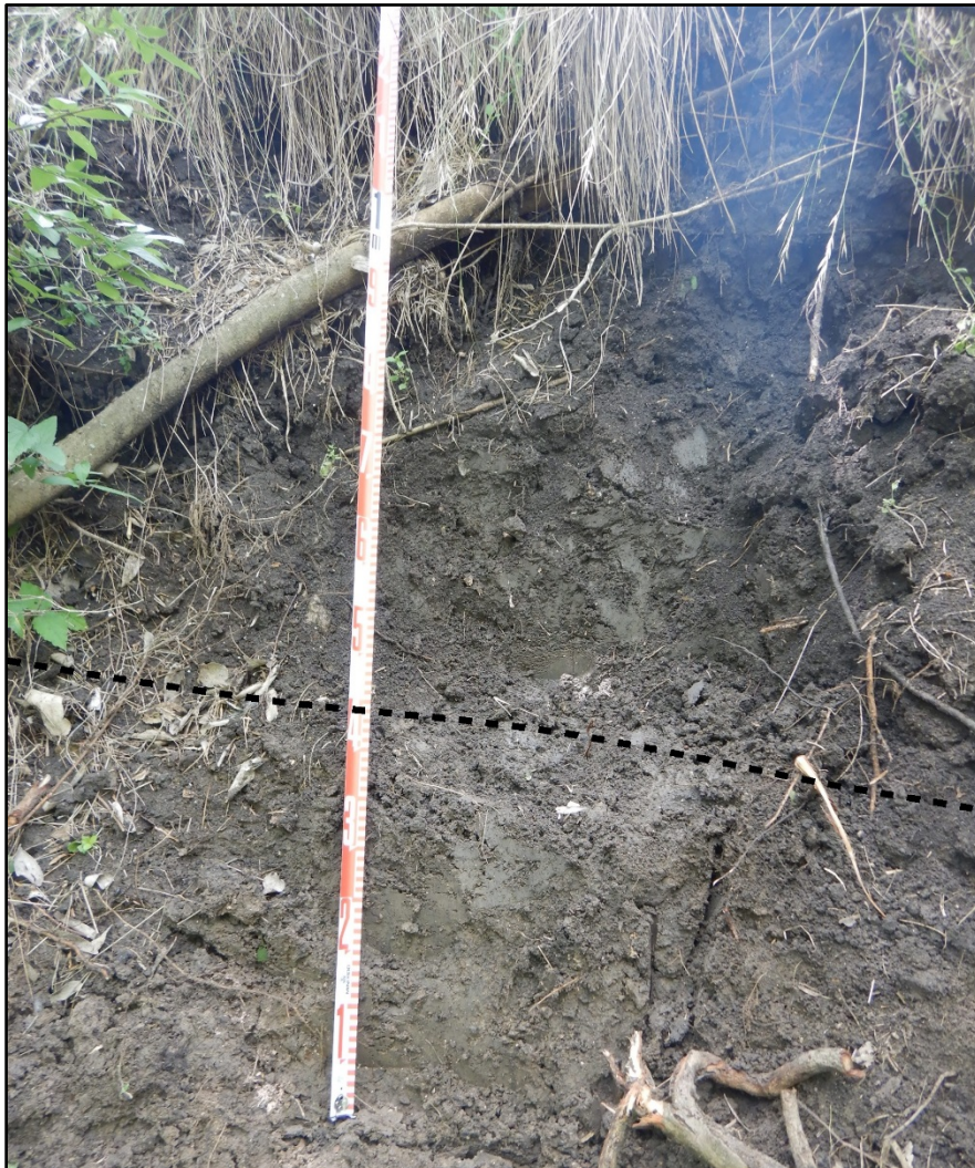
Figure 15. Photograph of a profile column of the south bank of the unnamed drainage. The dashed line delineates darker clay soil in upper column from lighter mottled clay beneath.
