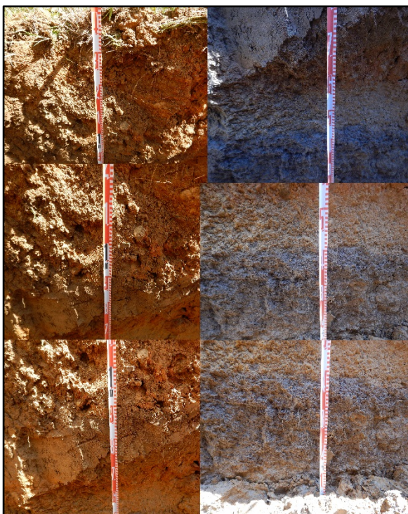
Figure 10. BHT1 north trench wall profile composed of overlapping photographs. The trench began to collapse before an adequate profile overview with scale could be taken.
