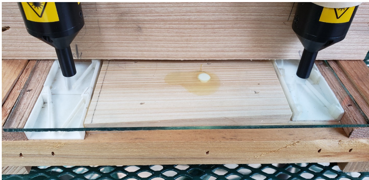
Fig. 3. Modified Bee hive entrances. Hives were fitted with bee escapes that allowed passage of bees in only one direction. Reader wands were positioned above these to scan tagged bees entering or exiting bee hives. A pane of clear glass allowed the transmission of the laser beam, but was thin enough to cause no interference with the radio transmission.
