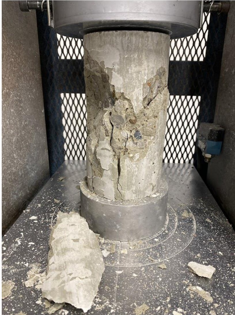
Figure 09. Batch 2 cylinder from WC curing condition on day 94.
