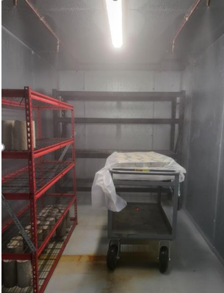
Figure 04. Batch 2 BCSA concrete cylinders placed inside the WR curing condition
