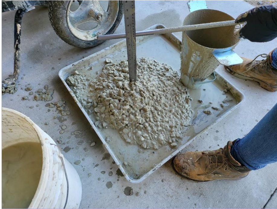
Figure 05. Concrete slump being measured after a slump test
