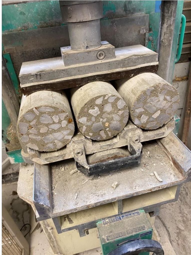
Figure 06. 3 cylinders in an end grinder with already-ground ends facing viewer
