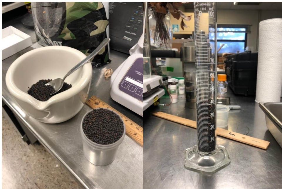
Caption: The seeds (pictured left) were used along with a graduated cylinder (pictured right) to measure the displacement and calculate the specific volume of the muffins.
