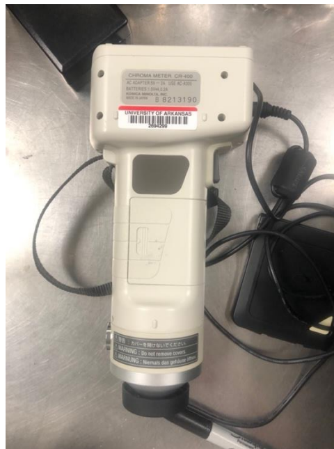
Caption: The Chroma Meter used to measure the color of the crust of the various muffins.
