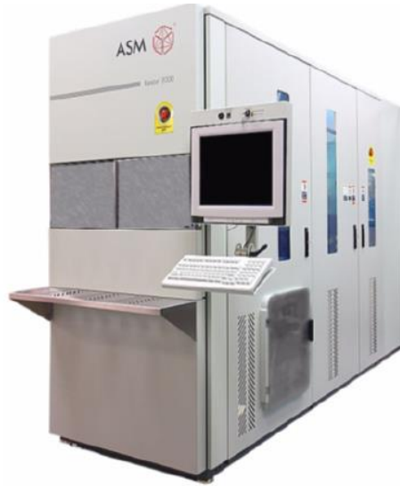
Figure 2.3. ASM's Epsilon® 2000 Plus reduced-pressure CVD assembly.
