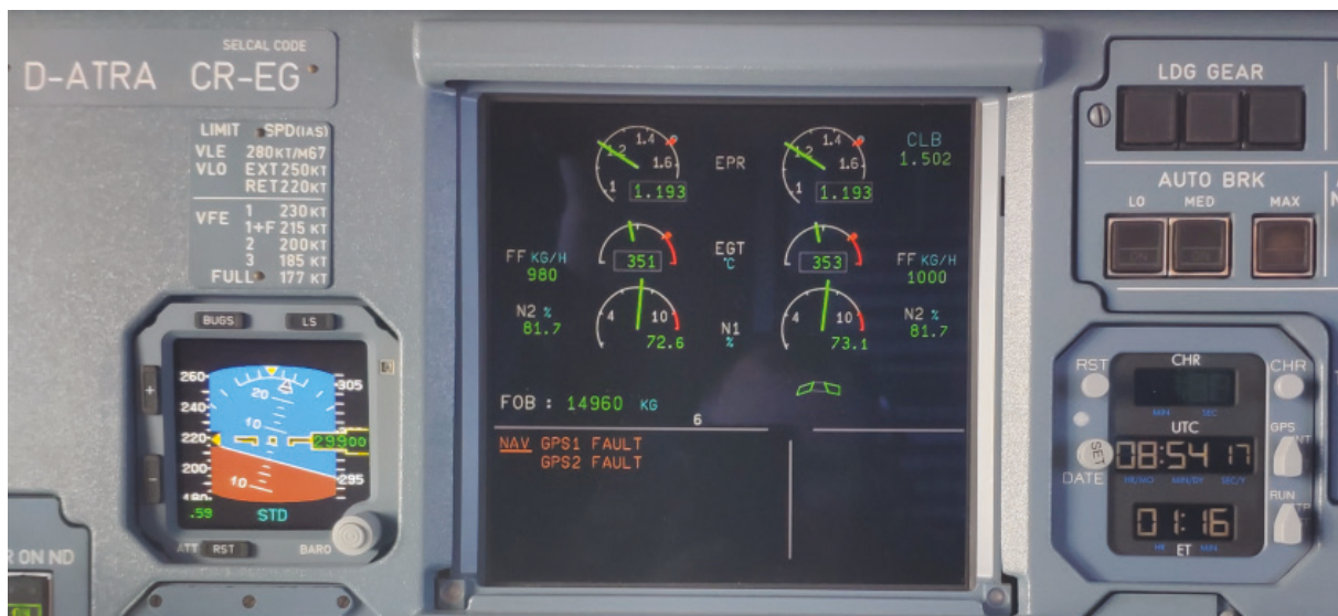
FIGURE 4 GPS 1 Fault and GPS 2 Fault refer to the GPS part of the two MMRs that operate independently of each other as part of the standard A320 avionics in D-ATRA. The error message suggests that both GPS receivers have failed, when in reality, they are operational but no useful GPS signal is available to them.
