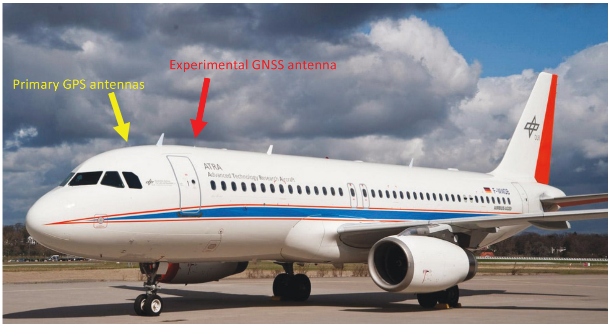
FIGURE 2 The cockpit is connected to two primary GNSS antennas providing GPS-only L1 signals. The experimental equipment is connected to the experimental GNSS antenna and captures L1, L2, and L5 from GPS, GLONASS, and Galileo.
