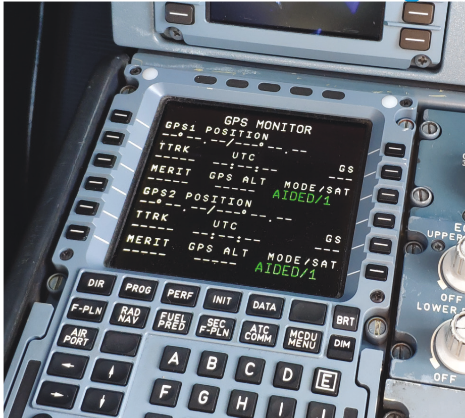
FIGURE 5 When the number of available satellites drops below four, the receiver goes into Aided Mode in which navigation avionics use the inertial platform to coast the navigation solution as primary position and velocity.
