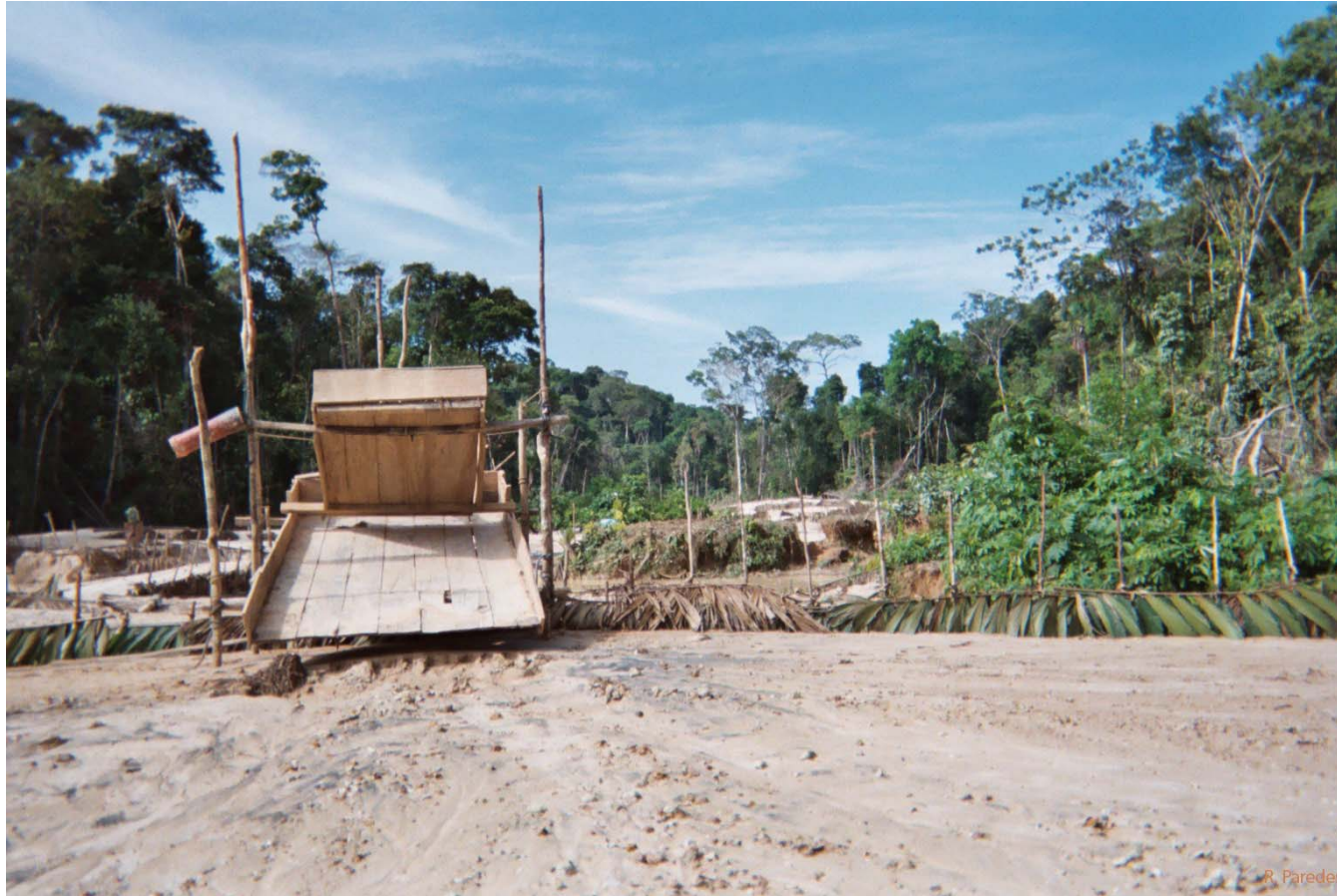
Figure 53. This filter uses a carpet (not shown) to catch the gold as it comes through the sluice. Behind the filter, palm fronds are used to separate the different holding ponds. Photo: Ronald Paredes del Águila.
