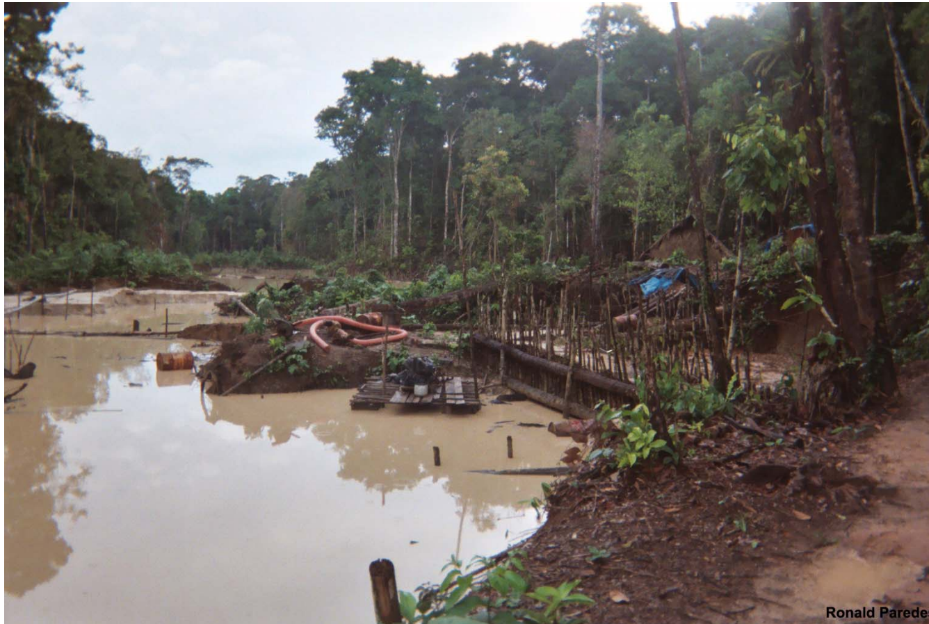
Figure 52. This holding pond is strewn with mining machinery and ringed by wooden wall supports. Notice the mining camp to the right. Photo: Ronald Paredes del Águila.
