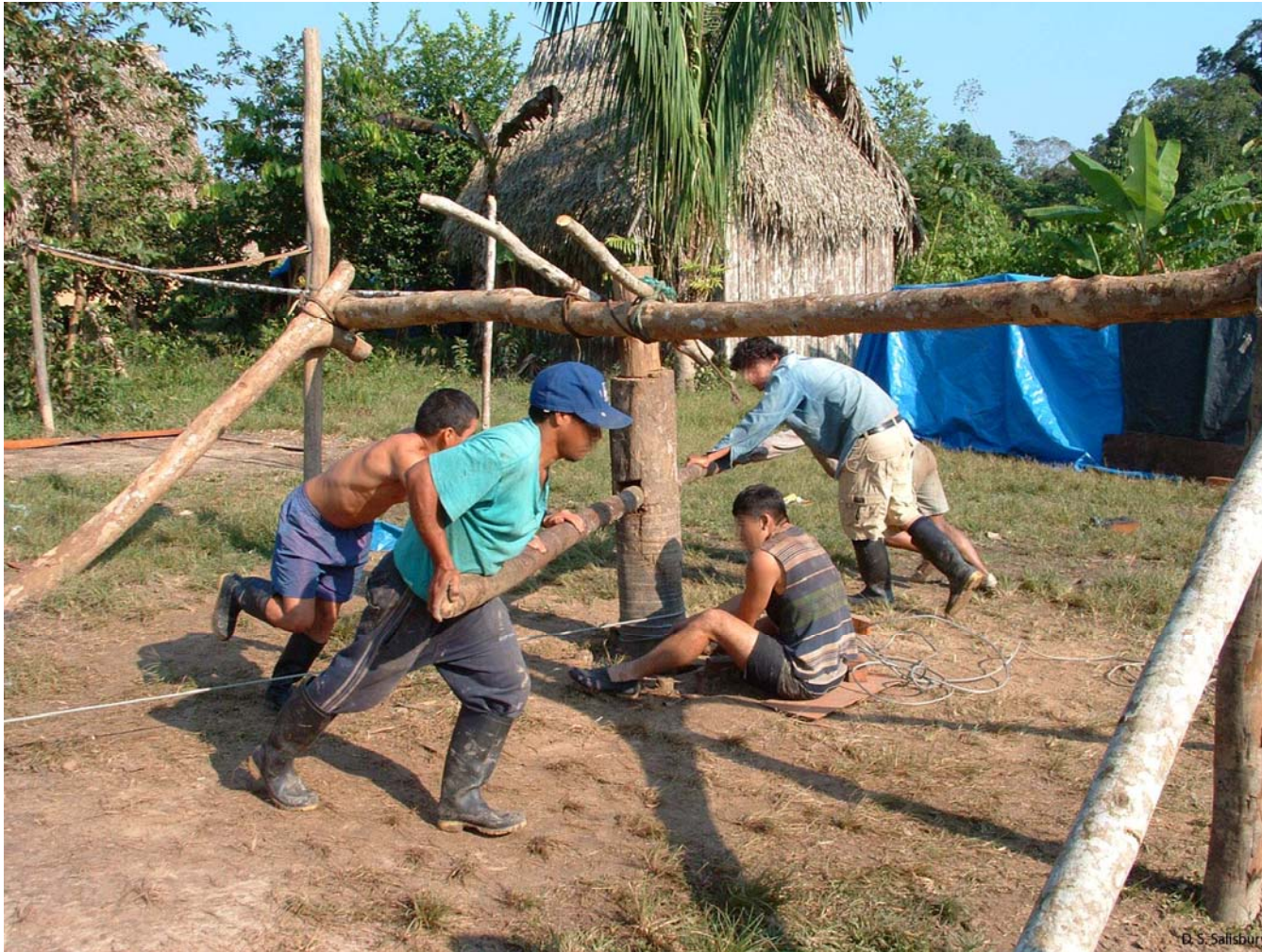
Figure 64. Loggers use a human powered pulley system to pull logs up the bank in borderland Ucayali.
