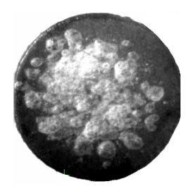
Figure 5.9: Semi-transparent JA2 propellant surface after exposure to plasma radiation during current study.
