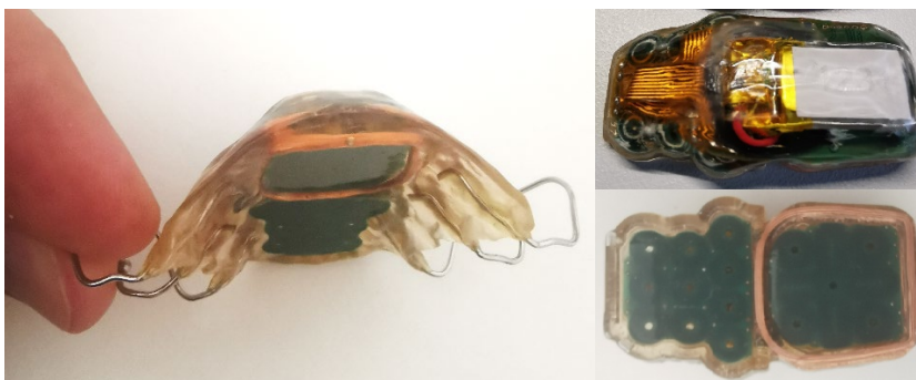
Figure 13- Left: The ITongue MPU custom made for a user. Right: The electronic core of the ITCI MPU
