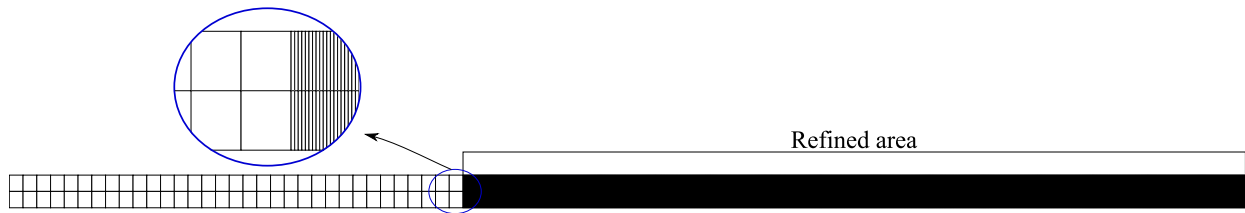
Fig. 13. Mesh of the reference model used for the performance and accuracy comparisons. Remark that the thickness of the specimen varies for some of the numerical tests.
