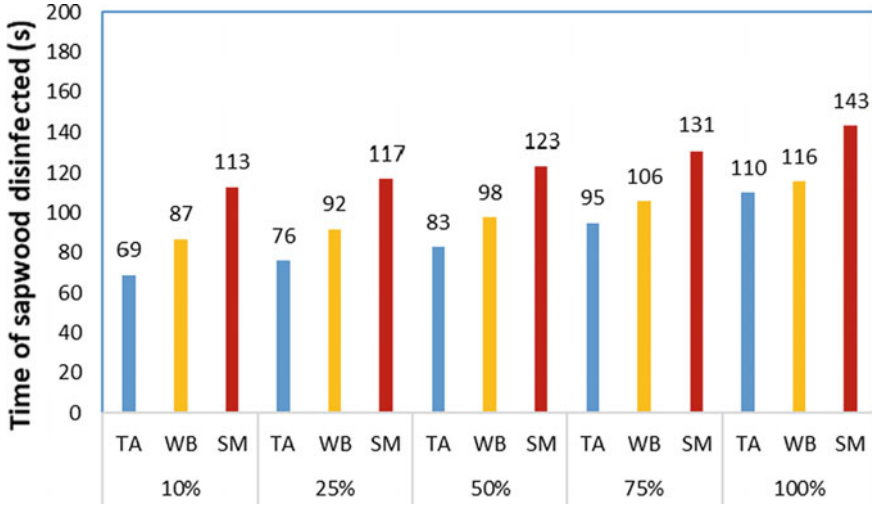
Fig. 14 Heat treatment by microwave energy ( I_0 = 1 \text{ W/cm}^2 , f = 2466 \text{ MHz} ): Evolution of percentage sapwood disinfected (initial temperature is 15 \text{ }^\circ\text{C} )
