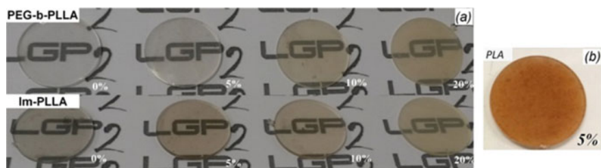
Fig. 7 Effect of adding various levels of modified surfactants onto PLA and injection molded into discs a and image of unmodified PLA composites (Mariano et al. 2017). Reproduced with permission from American Chemical Society through open access publishing
