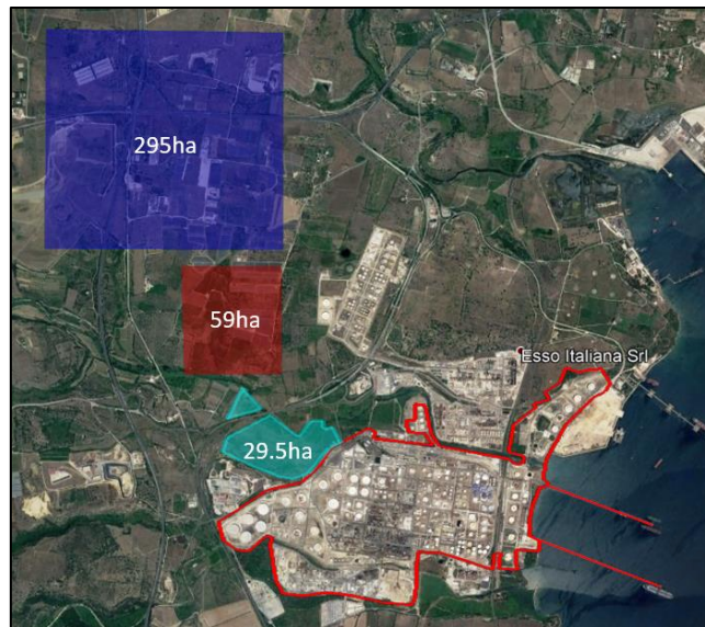
Figure 7: Light blue: land areas suggested as available by the refinery for the installation of renewable energy technology (S1 scenarios). Red: land area with twice the extension as the first (S2 scenarios). Dark blue: land area with ten times the extension of the first (S3 scenarios).
