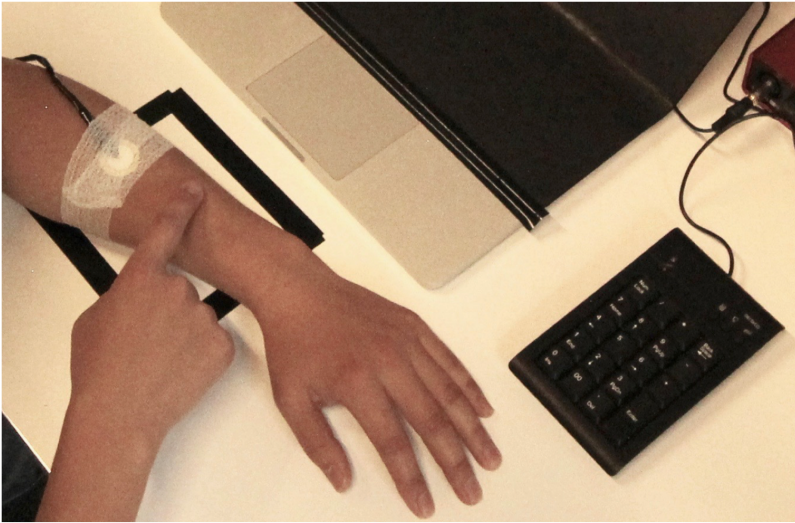
Fig. 4. Setup for the three input conditions: Skin, Touchpad, and Button. The input interface was always brought in front of the subject on a designated area (the black rectangle marked on the table). A separate screen displayed the interface and the Libet Clock. On the image, the Skin interface is shown.
