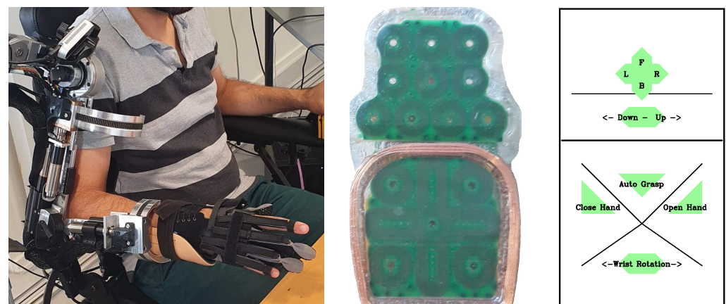
(a) The EXOTIC upper limb exoskeleton with a camera at the shoulder joint.
