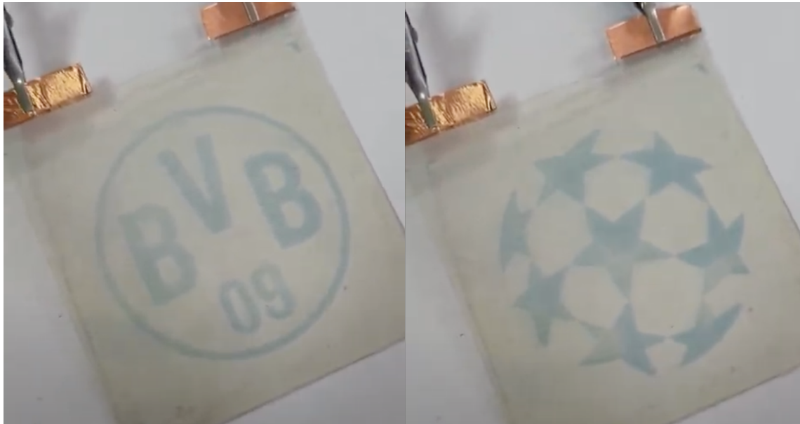
Fig. 2. Application of EC display with two different states, that allow to switch e.g. a logo, created in [7].
