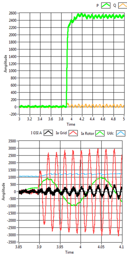
Fig. 22. Active power jump 0 to 2.5MW.
