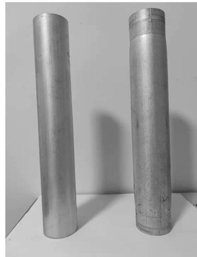
Fig. 6. Illustration of the initial and deformed 5049-O aluminium tubes in hydraulic bulge test with fixed end-condition.
