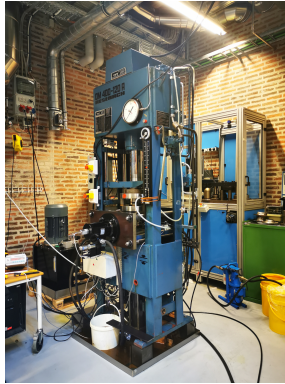
Figure 1: Experimental setup for tube hydraulic bulge test
