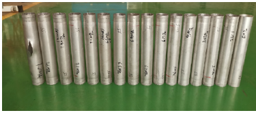
Fig. 9 Tubular specimens before and after hydraulic test.
