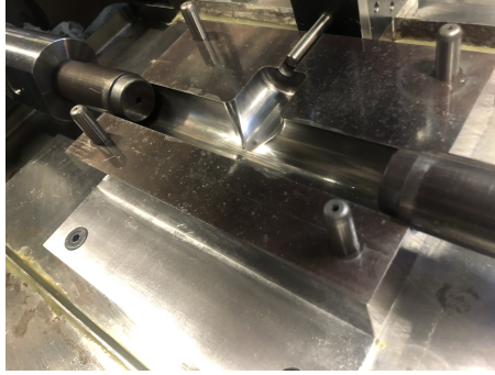
Figure 2: Dies and axial punches in experimental tools
