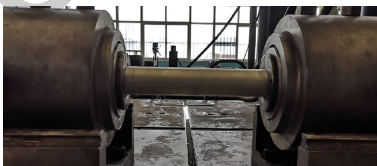
Fig. 8 Locking system for ends of tubular specimens on machine.
