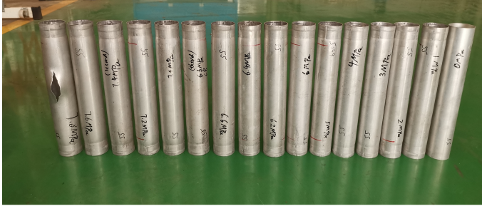
Figure. 7.1. Hydro-bulged tubular samples at multiple pressure levels.
