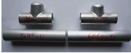
Figure 11: Hydro bulged specimens before and after test for aluminium alloys 5049-O and 6060-O
