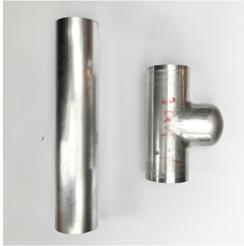
Figure. 7.2. Tubular sample before and after T-shape hydraulic bulge tests.
