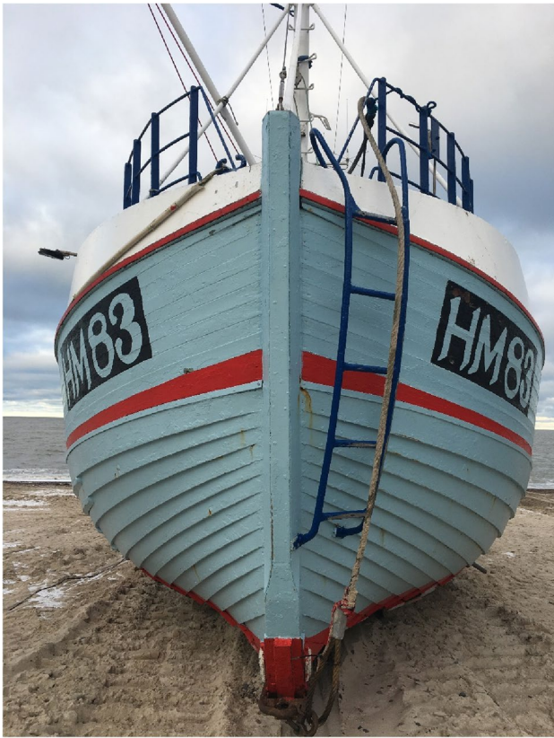
Fig. 3 Close up of a clinker built boat, showing the form of the sides of the boat, with the overlapping planks. Only an experienced individual can make the sides appear this even—and it is impossible to make the sides truly symmetrical
