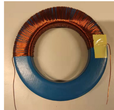
Fig. 10. Photograph of Prototype B: R102mm/65.8mm/15mm N87 toroid inductor.
