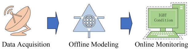
FIGURE 4 Steps of insulated gate bipolar transistor condition online estimation
