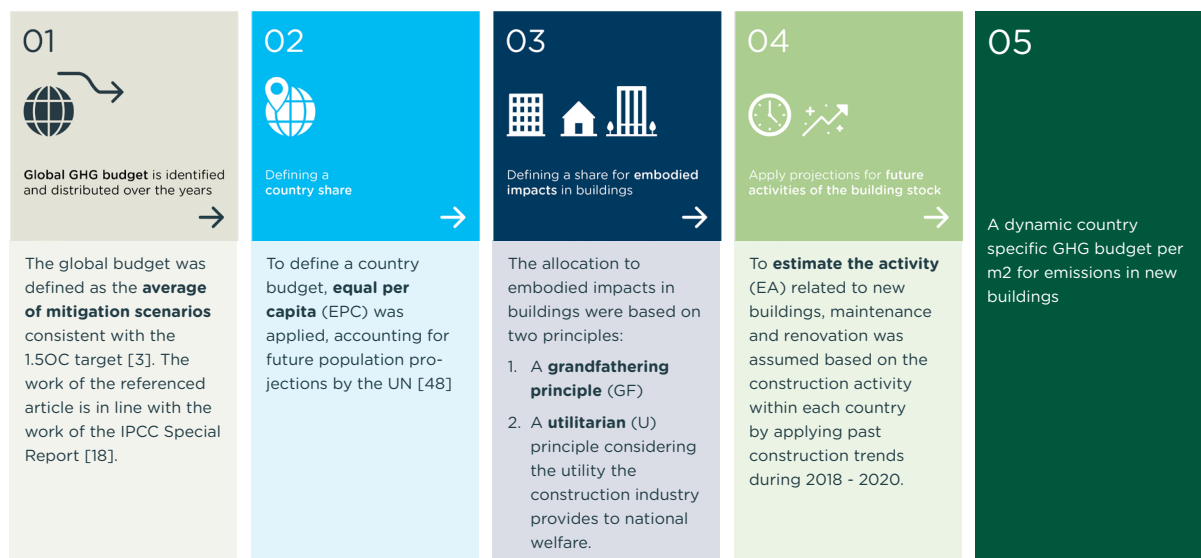
Figure 7: Approach to top-down carbon budget pathways for embodied carbon
