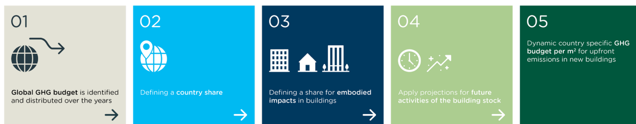
Figure 1: Downscaling from global budget to embodied carbon in buildings - a concept to set targets for embodied impacts in new buildings per m 2 .
