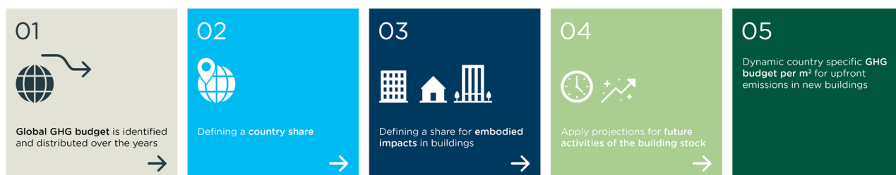
Figure 7: Downscaling from global budget to embodied carbon in buildings - a concept to set targets for embodied impacts in new buildings per m 2 .
