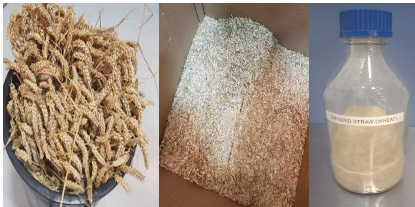
Figure 6: From raw form to fine powder- wheat straw for HTL experiments.
