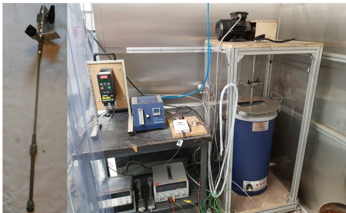
Figure 4: A coupled micro-batch reactor [On the left side], and the fluidized sand bath (Techne, SBL-2D) facility used for the HTL experiments [on the right side].
