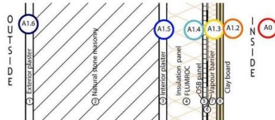
figure 51: Monitoring system: construction's temperature ©Eurac
