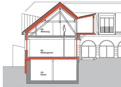
figure 119: Scheme insulation, cross section
