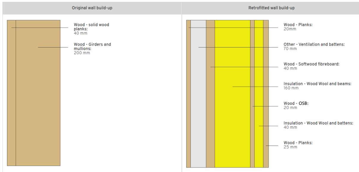
figure 170: Cross section before and after the intervention
