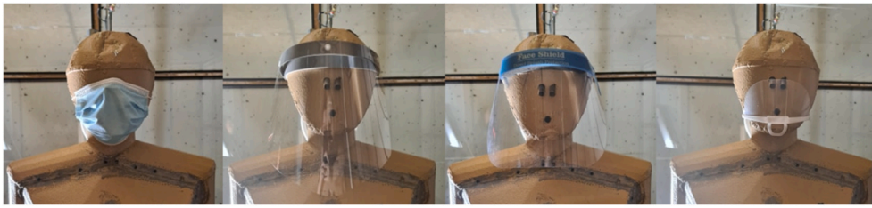
Fig. 4. Four types of PPE worn by the source manikin (a) Surgical mask (b) Open face shield (c) Closed face shield (d) Mouth visor.
