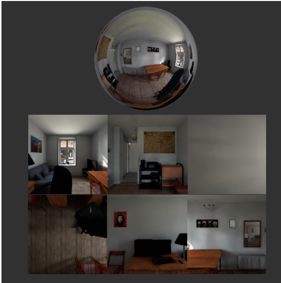
Figure 3: A reflection probe from the environment. Top part is the probe itself, with the bottom part being the cubemap.
