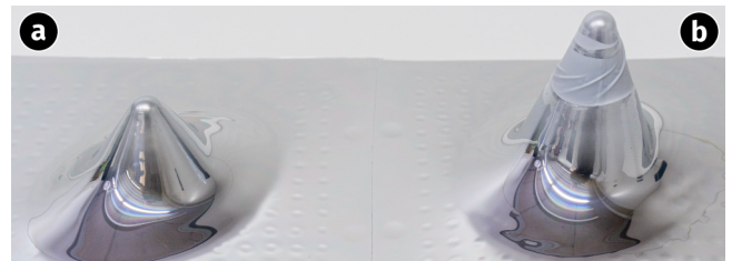
Figure 13: Stress test to achieve rupturing of the metallization layer during vacuum forming. a) 40x50mm cone b) 60x50mm cone.
